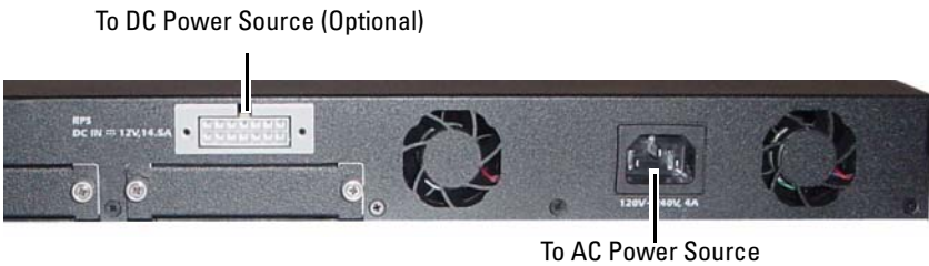
Figure 1-15. AC and DC Power Connection to Switch
